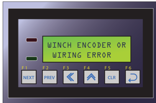
Figure 7: Winch Encoder or Wiring Error Message
