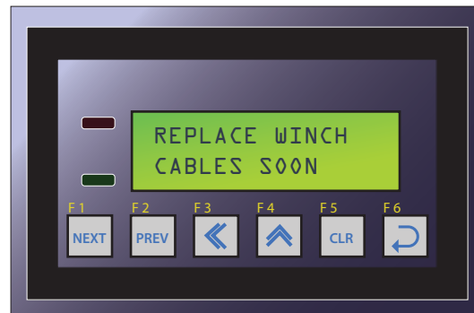
Figure 6: Replace Winch Cables Soon Message
